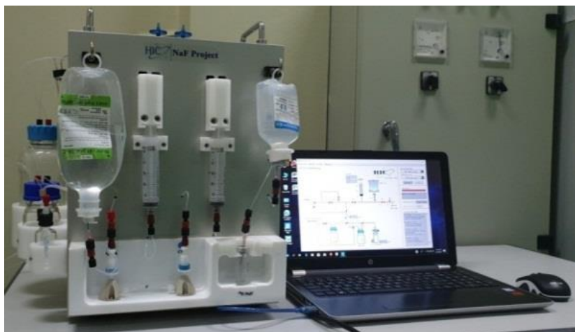
Fig. 2. A view of the home-made automatic module used for preparation of ^{18}\text{F} -NaF
