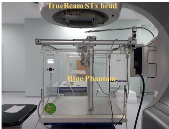
Fig.1. Photograph of Blue Phantom (IBA, Germany) scanning water phantom below TrueBeam STx head in the experimental setup.
