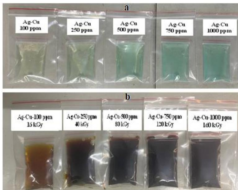
Fig. 1. Ag-CuNPs samples with total Ag<sup>+</sup> and Cu<sup>2+</sup> concentrations of 100–1,000 ppm, (a) before irradiation; (b) after irradiation
