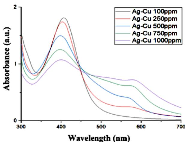
Fig. 2. UV-Vis spectra of Ag-CuNPs solutions with total Ag<sup>+</sup> and Cu<sup>2+</sup> concentrations of 100–1,000 ppm
