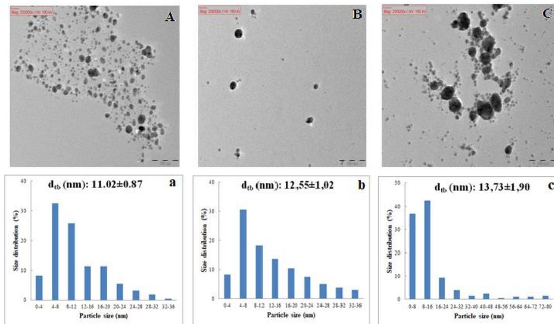
**Fig. 3.** TEM images and size distribution of Ag-CuNPs with total  $\text{Ag}^+$  and  $\text{Cu}^{2+}$  concentrations of 250 (A,a), 500 (B,b) and 1000 ppm (C,c)
