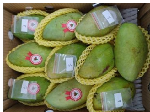
Fig.2. Carton boxes of Hoa Loc mango with the positions of B3 film dosimeters
