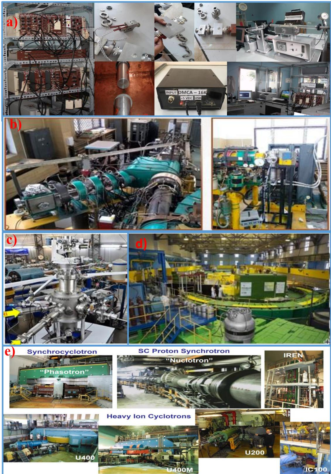
**Figure 1.** a) Positron annihilation laboratory at CNT (Vinatom). From b) to e) Nuclear analytical facilities at JINR (Dubna): slow positron beam accelerator (b), Rutherford back scattering spectroscopy (c), neutron sources from IBR-2 reactor used for neutron diffraction measurement (d), and ion beam accelerators (e). Figures b-e) are taken from [26].
