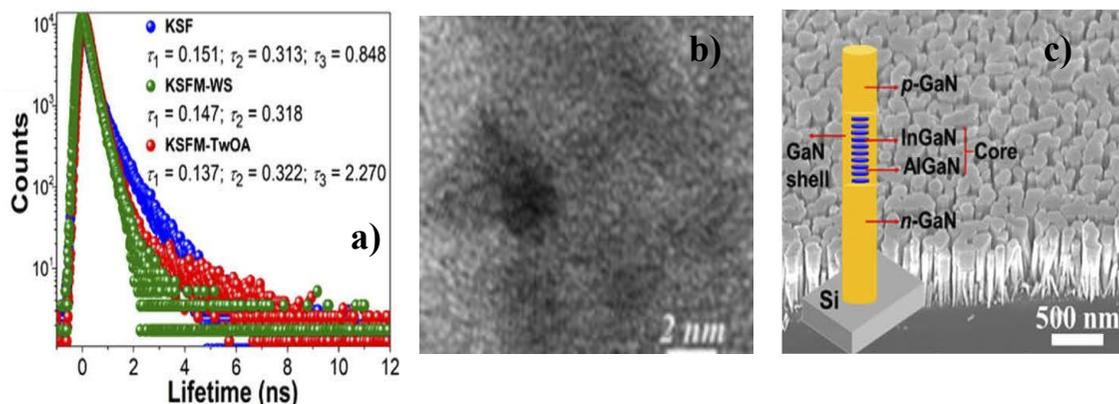
**Figure 4.** a) PAL spectra of the KSF, KSFM-WS and KSFM-TwOA nanocrystals. b) HRTEM images of KSFM-TwOA. c) A 45° tilted SEM image of the nanowires on silicon wafer. Inserted image shows the schematic structure of an InGaN/AlGaN core-shell single nanowire LED. Adapted from [17].
