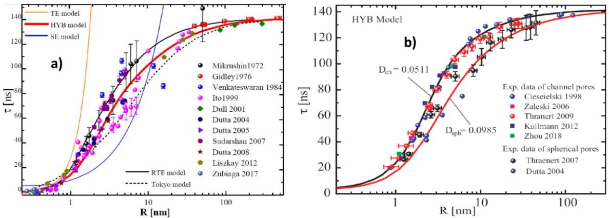
**Figure 2.** a) The *o*-Ps lifetimes obtained within the TE, SE, Tokyo, RTE, and HYB models versus the experimental data for different porous materials. b) The *o*-Ps lifetimes obtained within the HYB models versus experimental data for the materials with spherical and channel pores. Adapted from [18].
