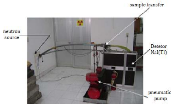
Fig. 4. Automatically sample transfer system.
