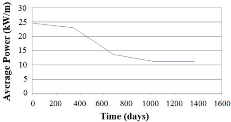
Fig. 2. The linear heat generation rate of the fuel rod during operation
