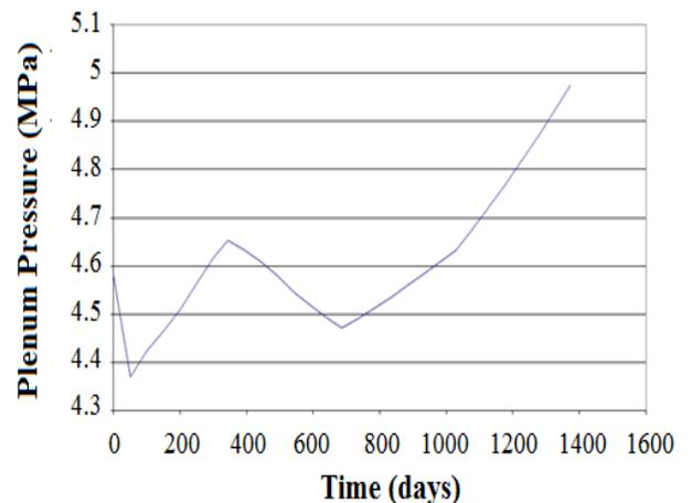
Fig 6. Rod internal pressure
