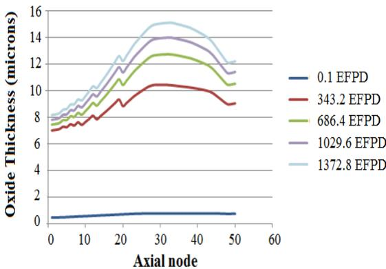
**Fig 14.** Cladding oxide thickness
