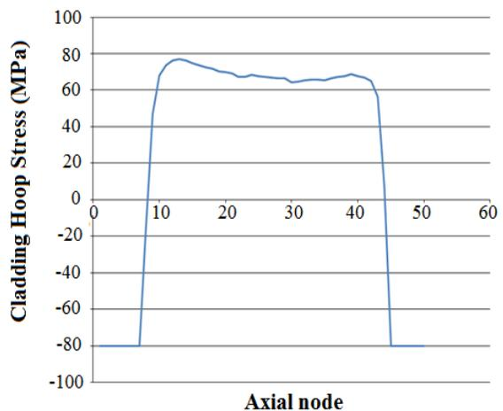
Fig 8. Cladding hoop stress
