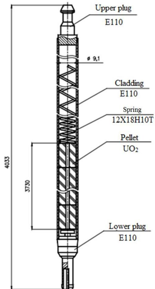
Fig. 1. Configuration of TVS-2006 fuel rod
