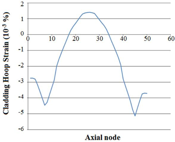
**Fig 9.** Cladding hoop strain
