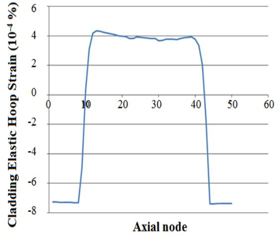
**Fig. 10.** Cladding elastic hoop strain
