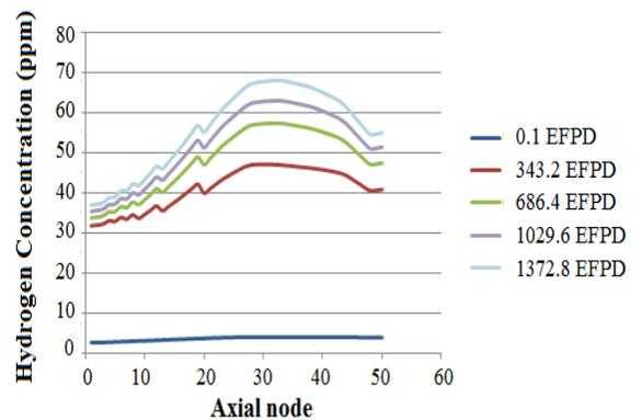
**Fig 15.** Claddinghydrogen concentration
