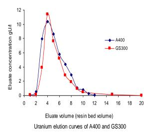
Results show that in the same condition, elution curves of GS300 and A400 resin are divided into two stages. In the first one, most of the uranium is eluted from the resin in about first 10 BV. Later stage, to elute the entire uranium, relatively large volume of eluant is needed. Elution process can be completed in 15-20 BV of eluate.
