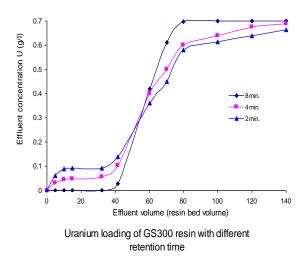
Experimental results show that, similarly to IRA-420, the sorption curve of two resins can be divided into three parts: first, most of the uranium is sorbed in resin beads so uranium concentration in effluent is very low and changes slowly. In the next section (after breakthrough point), uranium concentration increase very fast. In the last section, uranium concentration varies slowly and resin beads reach state of uranium saturation.
