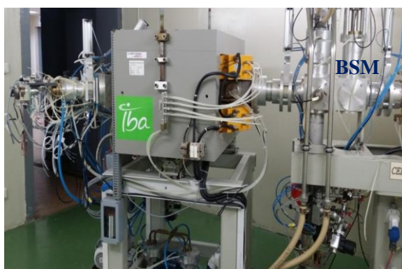
Fig.1. The Beam Selection Magnet located at the end of the beamline
